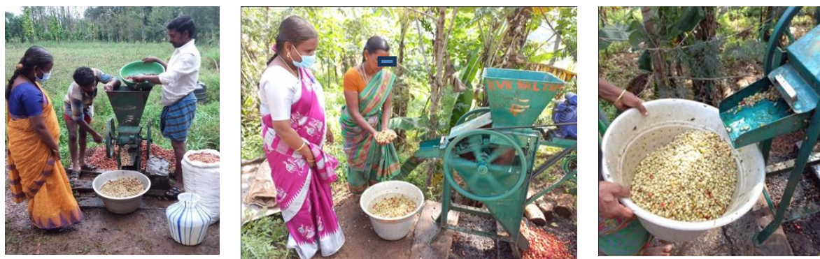
Fig. 8. Pulping of coffee beans by using electrically operated mobile coffee pulping machine
