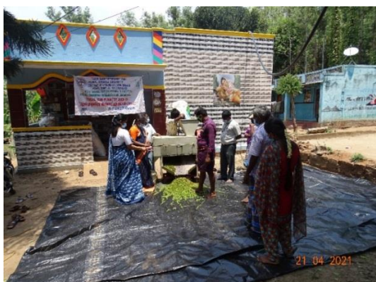
Fig. 1. Pepper threshing by using electrically operated pepper threshing machine
